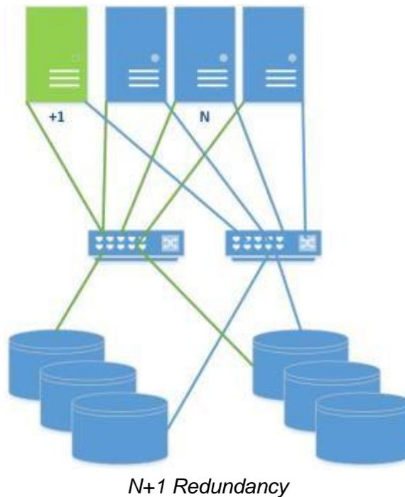
At the network level, similar N+1 design provides for multiple network interfaces to connect with multiple redundant network switches to multiple networks for a completely redundant path should any single component or system fail. Of course, all power to these "outside the host" networking systems is redundant. All of these systems are again, N+1.
